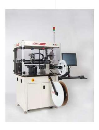
The TM 500 is a multiple input pick and place test, inspection and taping machine designed for high mix/low volume production environments for electronic devices.
